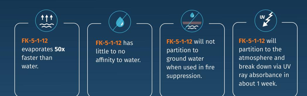
**FK-5-1-12** is not on the EPA TRI list (Toxic Release Inventory). **FK-5-1-12** is listed on the EPA SNAP list as safe for use in occupied spaces.
